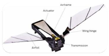
Figure 6. Robot Fly
