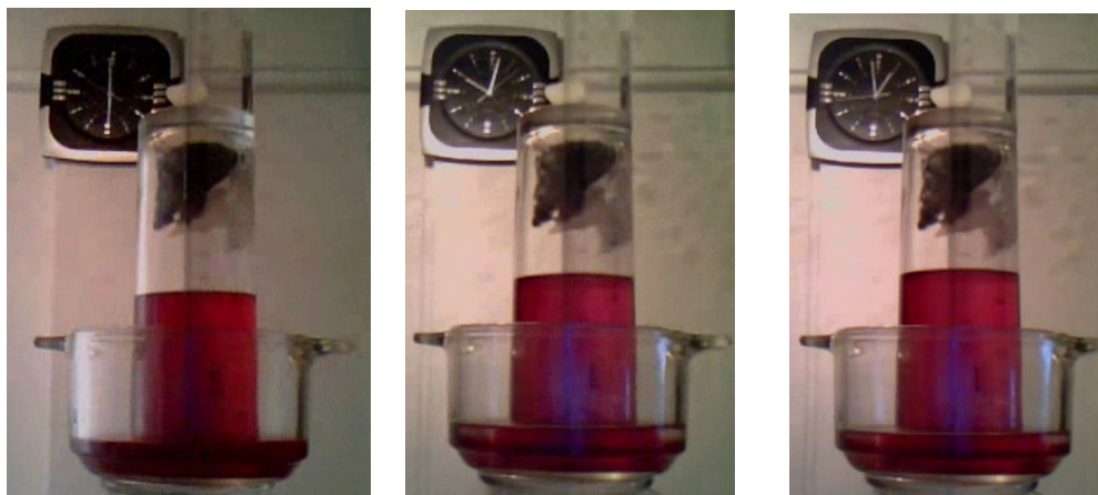
Fig. 2. Absorption of Oxygen by Iron wool in the air trapped by the colored water
