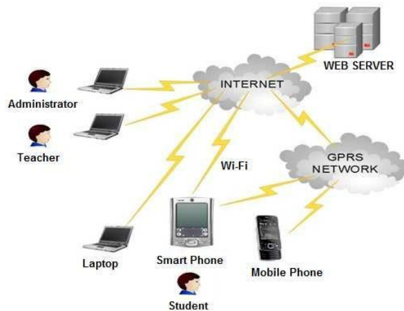
Figure 1: Mobi – Exam system structure.
