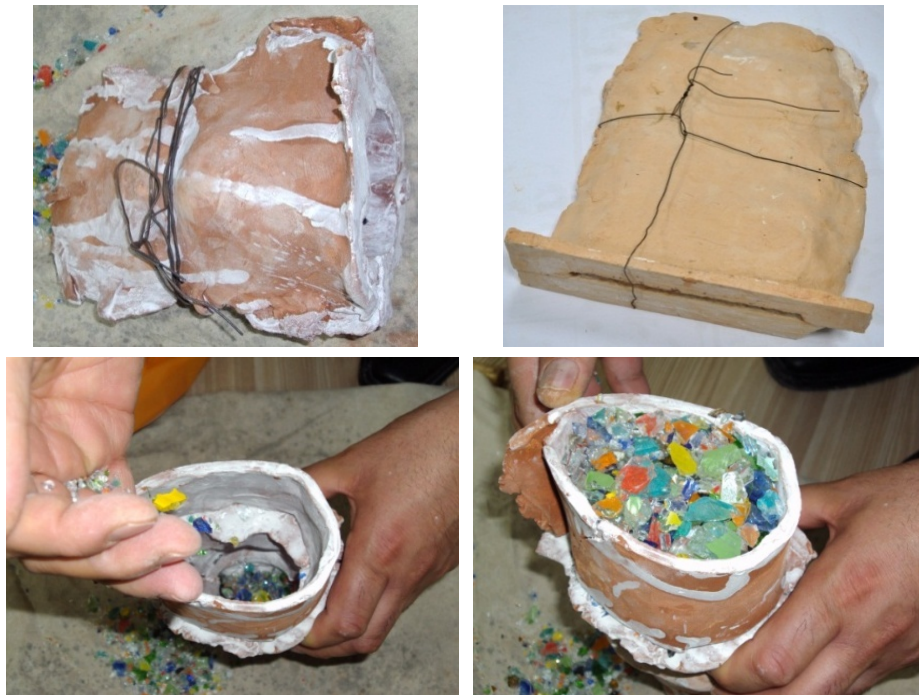
Photograph 10. Tying the Chamotte Mould with String and Filling It with Glass
