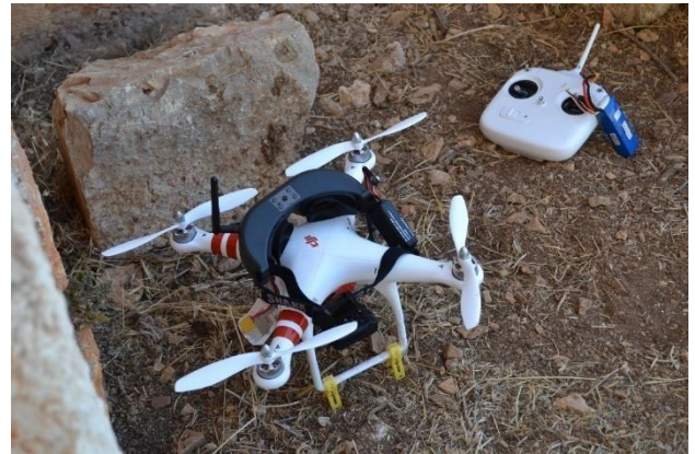
Figure 11. UAV, FPV control and image transfer system
